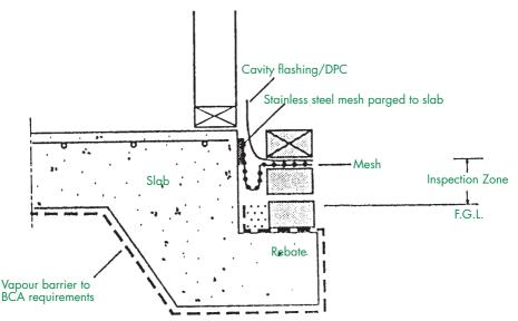
The mesh is parged (bonded) to the side of the slab rebate, stepped down into the cavity and generally run on the second course of the outside brickwork below the flashing or dampcourse.
